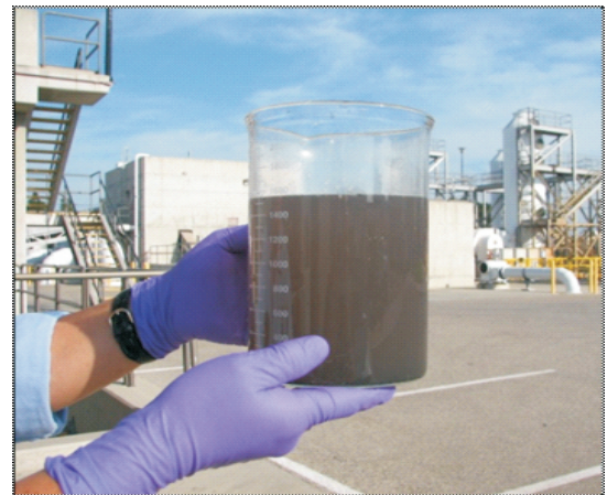
A wastewater sample after preliminary treatment.
