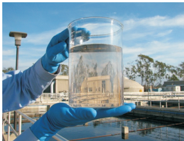
A wastewater sample after secondary treatment.
