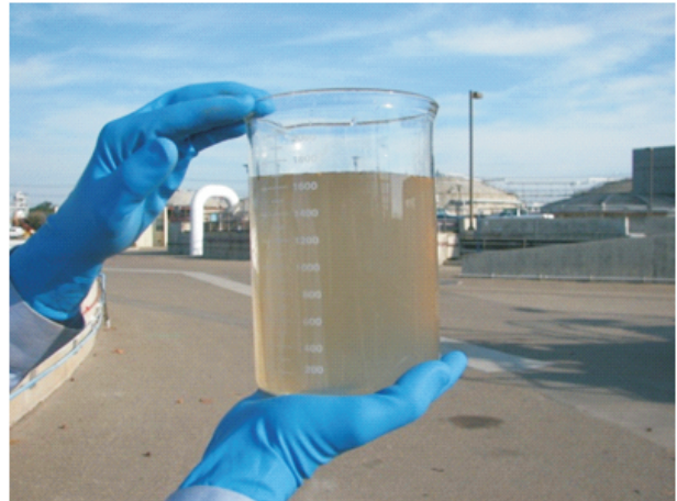
A wastewater sample after chemically enhanced primary treatment.
