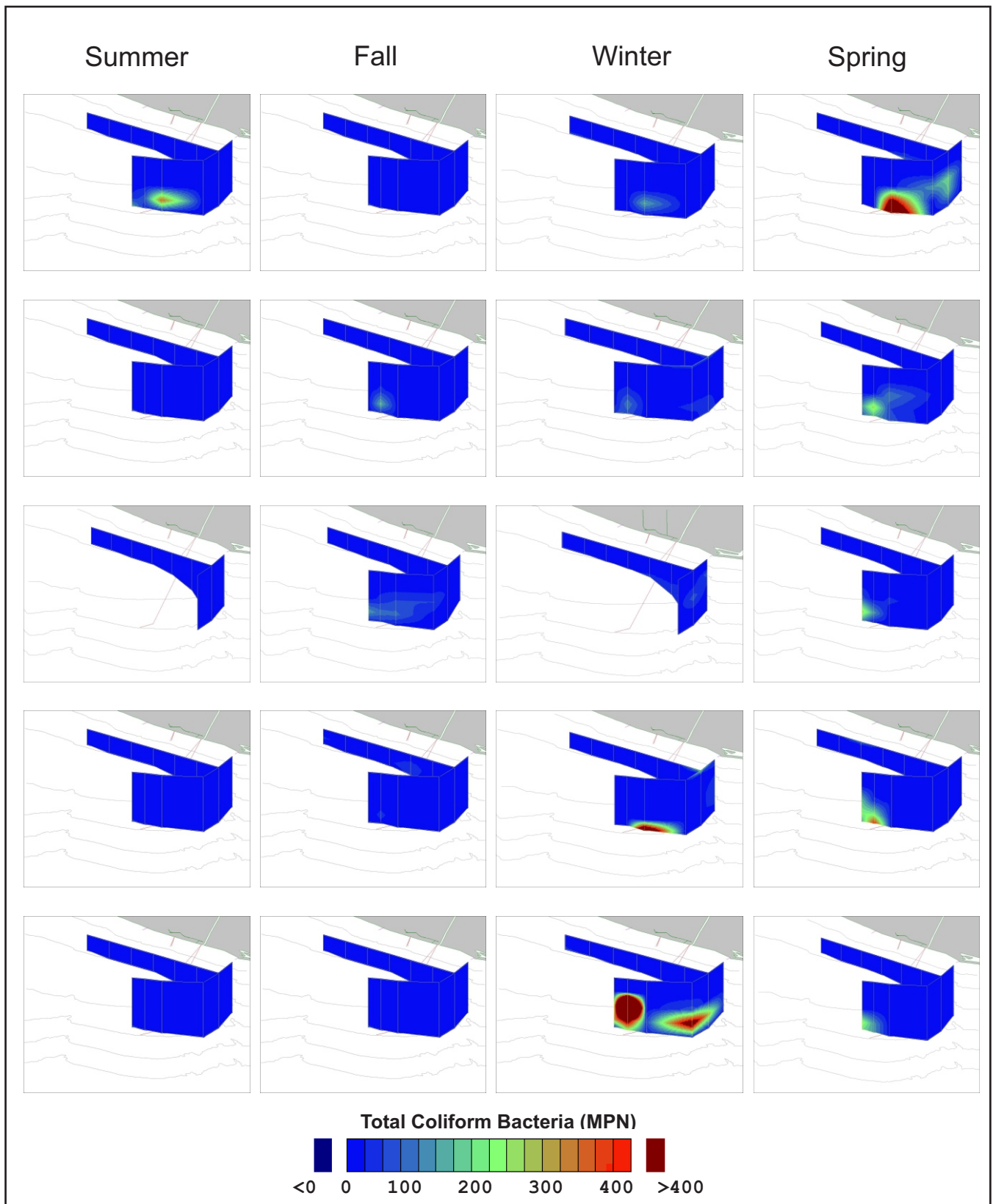
Figure 3-27. Seasonal patterns of total coliforms (MPN/100mL) for summer (July 26, 27, August 9, 10, 22), fall (October 27, November 2, 3, 8, 9), winter (February 7, 9, 15, 16, March 7, 2012), and spring (April 18, May 2, 3, 8, 10).
